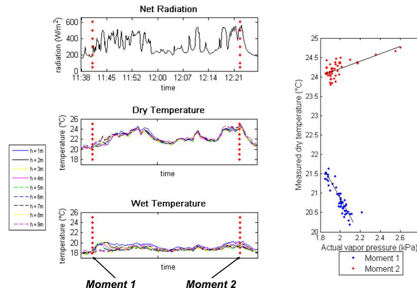
Observed net radiation and dry and wet temperature between 1m and 9m above ground surface over time.
